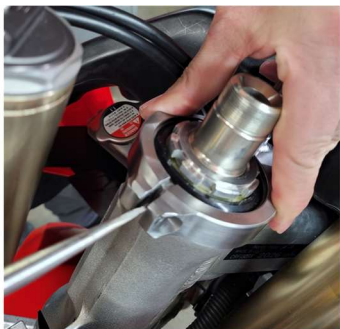
Remove bolt & spread bracket to install
