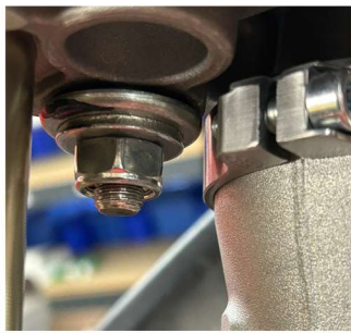
Be sure the lower cone clears the frame bracket at full lock on the underside of the triple clamp.
