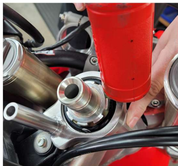
Tap bracket down until securely flush
