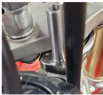
Note how close the cone and nut are on the underside but do not touch.
