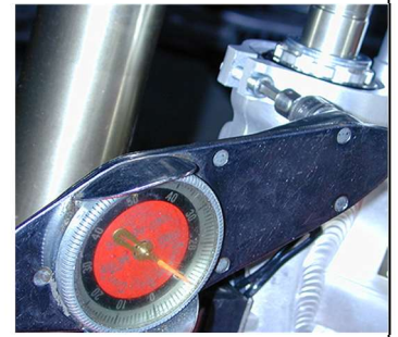
Torque the frame bracket pinch bolt to at least 96-108 inch lbs., or the equivalent of 8-9 foot lbs.
